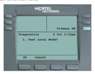
Test local mode transitions the terminal to its S2, for registration with a Survivable Remote Gateway.
